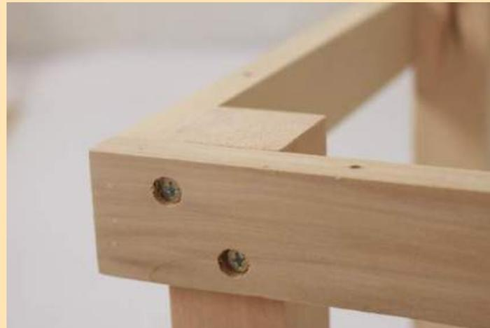
Attach the leg assembly to the bottom of the bench surface. Choose which surface of the bench you prefer to be the top and bottom.
