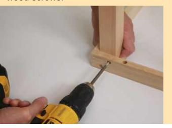
Ensure that the legs' ends are flush with the bottom edge of the frames
