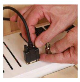
Attach the 'D-Sub' computer style connector as shown.
